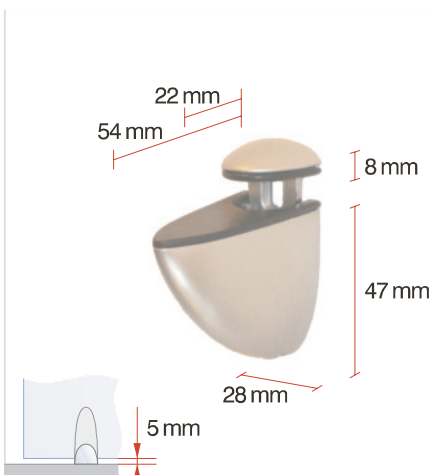
glass shelf bracket, adjustment range 0-20 mm
